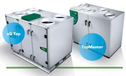
**The eQ Top** is a compact air handling unit, manufactured in two sizes with an air flow range up to 1,6 m³/s. The eQ Top is a flexible air handling unit, which is easy to install and commission. The unit is supplied with direct-driven supply and extract air fans, supply and extract air filters and a rotary heat exchanger. There is a wide range of accessories for the eQ Top for in-duct air processing. This range includes everything necessary such as dampers, coils, silencers etc.
